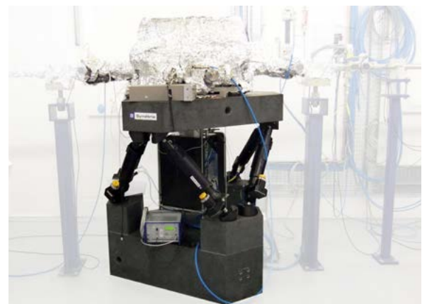
JORAN hexapod has been developed in collaboration with ESRF synchrotron to position mirrors with very high resolution.
