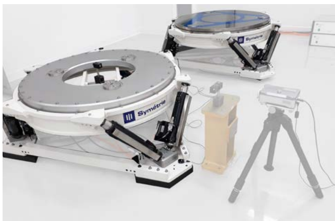
Customized JORAN hexapods with extra R_z rotations calibrate the segments of the primary mirror of ESO ELT telescope at Safran REOSC.
