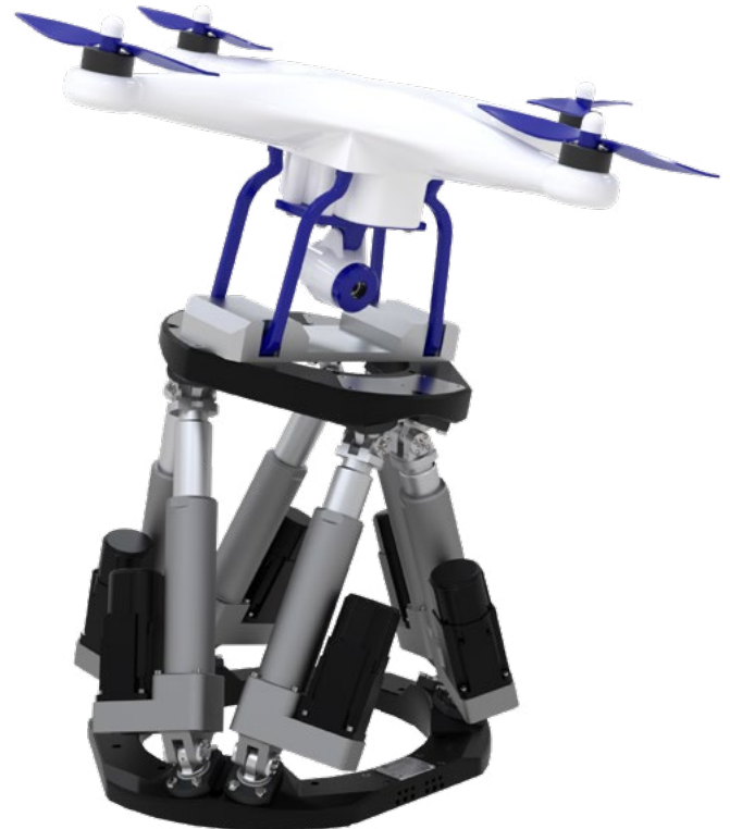
HEGOA hexapod with a drone equipped with a camera to test the reactions of the system during flight movements.
