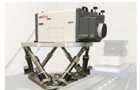
This ZONDA hexapod positions a laser interferometer (Zygo) in order to characterize the X-ray mirrors at Synchrotron SOLEIL.
