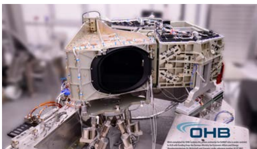
This ZONDA S hexapod aligns two parts of a space telescope in an ISO5 clean room.
