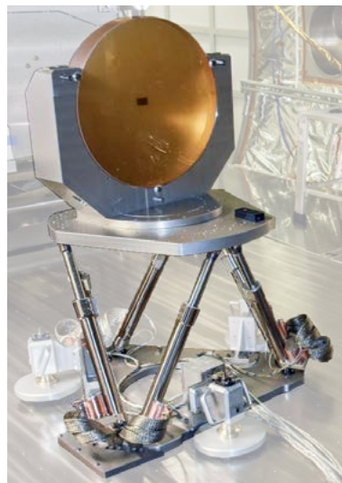
ZONDA Hexapod in a vacuum chamber with a mirror for optical calibration at Thales Alenia Space.
